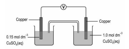
At room temperature, she found that the initial voltmeter reading was +0.16v.
